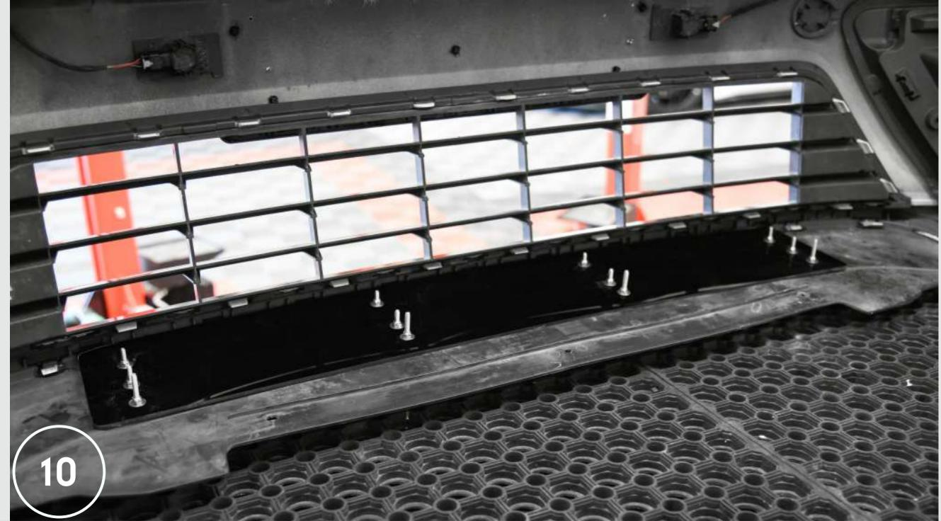
6. Drill through the original holes in the splitter to open through the bumper and the reinforcing insert.
