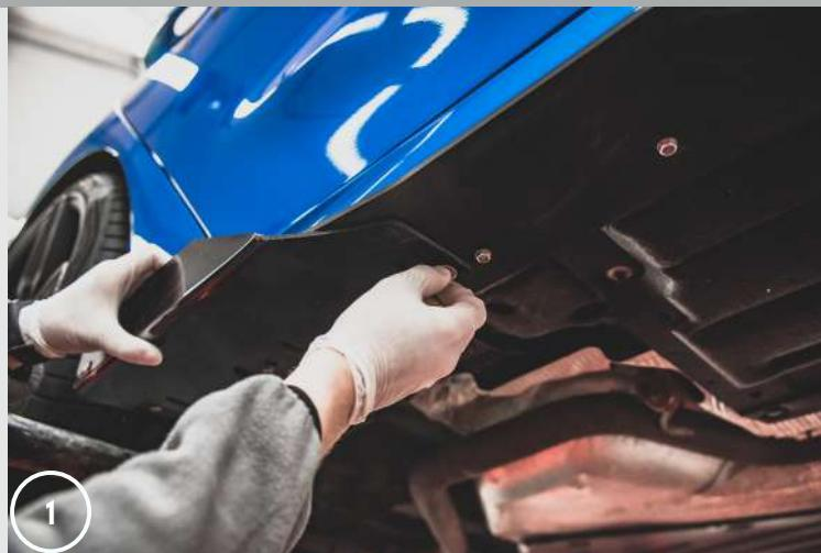
2. Using a bolt with a washer, lightly attach the flaps to the splitter so that it is possible to move the flaps.
