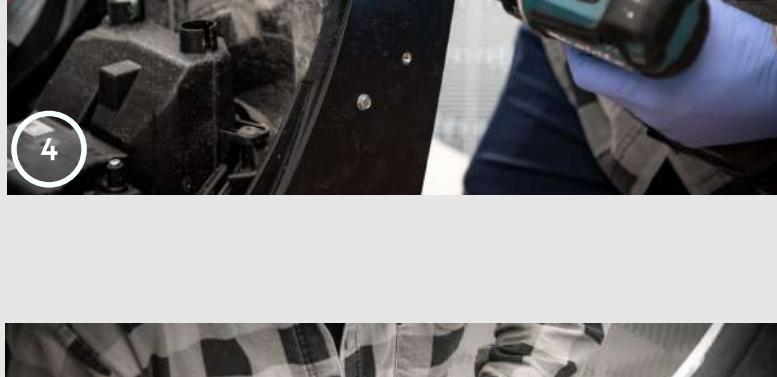
4. Drill the bumper in places consistent with the splitter holes.
